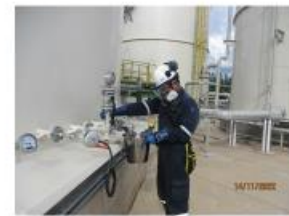
4. First sampling (May have stand to prevent chemical spill while open valve)
